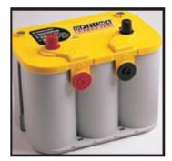
Battery Model: YTU 4.2 Part Number: 814 254 000 888 2 Nominal Voltage: 12 volts NSN: 6140 01 457 4341 Description: High power, dual purpose engine start and deep cycle, sealed lead acid battery
